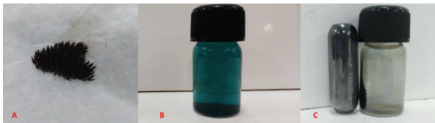
Fig. 1 a Magnetic adsorbent, b magnetic adsorbent in dye solution, c easy separation of adsorbent material after the application part
